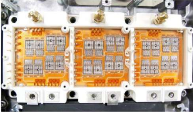
Figure 32: 2016 BMW i3 Infineon inverter power module. Source: DOE Office of Energy Efficiency and Renewable Energy, FY 2016 Annual Progress Report for Electric Drive Technologies Program , July 2017.
