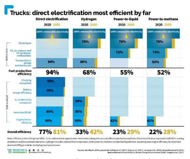
Figure 7: Conversion efficiencies of the different vehicle technologies
